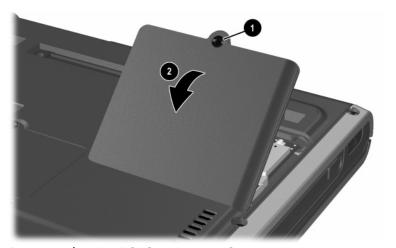
Removing the Mini PCI Compartment Cover
